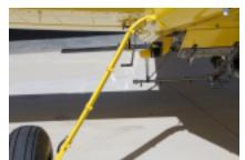
design to create a safer platform for both plane and pilot. The blade has been heat treated to a level of 61 Rockwell Hardness which would be equal to the hardness of a file or chisel. Spacer blocks have been positioned at five points along the blade to increase strength and stabilize the blade in case of a wire strike. Adel clamps positioned along the trailing edge of the landing gear secure the brake line and do away with the standard black zip ties currently used to secure the brake line.
